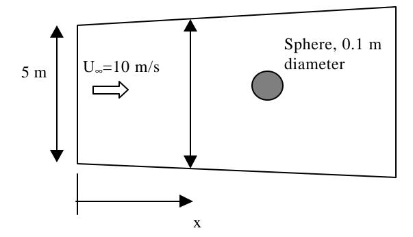
Solution: In order to maintain a constant velocity inside the tunnel, the tunnel wall has to be displaced outward in order to accommodate the growth of the boundary layer. The mass flow displaced by the presence of the boundary layer can be related to  $U_{\infty}d^*$  by the definition of the displacement thickness. Therefore, the tunnel height has to be  $H(t)=5+2d^*(x)$ .
