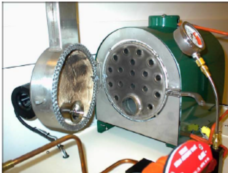
Figure 3: The boiler (open). The flame burns in the large pipe and the hot combustion gas returns through the smaller pipes to the exhaust chimney. The burner is mounted on the door. The lower part of the boiler contains liquid, the upper part contains steam. The upper pipes are surrounded by steam, which can be superheated.
