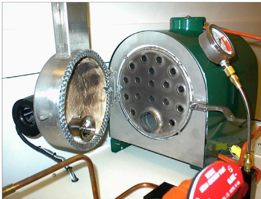
Fig. 3: The boiler (open). The flame burns in the large pipe, and the hot combustion gas returns through the smaller pipes to the exhaust chimney. The burner is mounted in the door. The lower part of the boiler contains liquid, the upper part contains steam. The upper pipes are surrounded by steam, which can be superheated.
