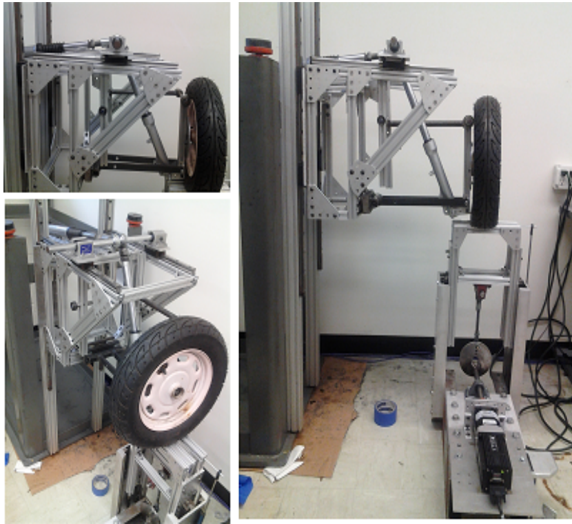
Figure 2: Quarter Car Experimental Setup
