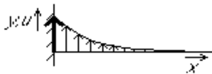
Figure 24.1: Viscous flow next to a moving plate
