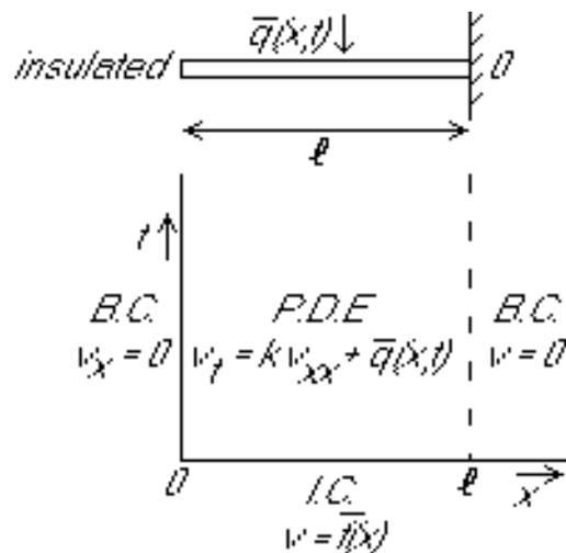
Figure 4: Heat conduction in a bar.
