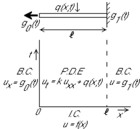
Figure 2: Heat conduction in a bar.
