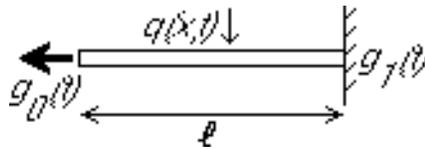
Figure 1: Heat conduction in a bar.
