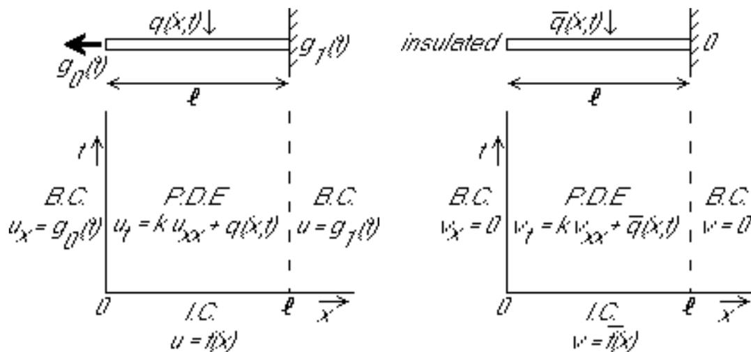
Figure 3: Heat conduction in a bar.
