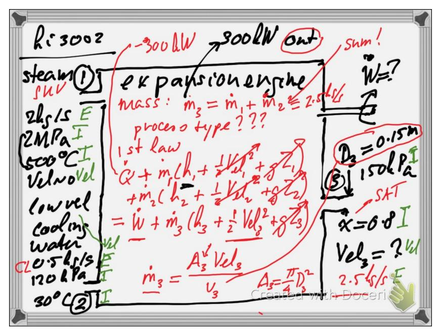
()SUV 2 MPa, 500°C h=? B.1.30 2000 LPA 500°C h=3 C.L. 2019a 300 - B.1.4X -> 30°C Satlig B.1.1 230°  $h_2 = h_f = 125.77 l)$ Sat 2P 150LPA, x = 0.88-1-2 (Sat) 2150 Pa line V1 = 0.00 1053 m3/kg U2=1.6828  $V_3 = V_4 + X_3 V_4 = 092767$  $k_{f} = 467.00$   $h_{fs} = 2226.46$   $h_{s} = h_{f} + 1 h_{s} = 22.40.25$
