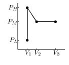
$$\frac{1}{2}(P_H + P_M)(V_2 - V_1) + P_M(V_3 - V_2) \qquad .$$
