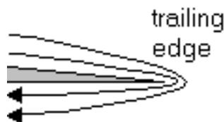
Viscous effects do not allow that. So we must make sure that the rear stagnation point deforms into the trailing edge. To make this easier, we will first rotate the flow so that the rear stagnation point moves to the point 1:
