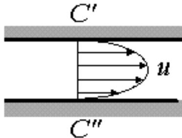
At and beyond station C the flow is called developed. We will assume that the flow is nonturbulent and that the streamlines have become parallel. These assumptions allow us to solve the incompressible Navier-Stokes equations exactly!
