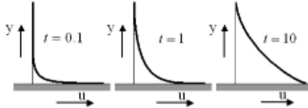
Supposed shape after scaling  $u$  with  $V_0$ , and  $y$  with a characteristic *boundary layer thickness*  $\delta$  that increases with time:
