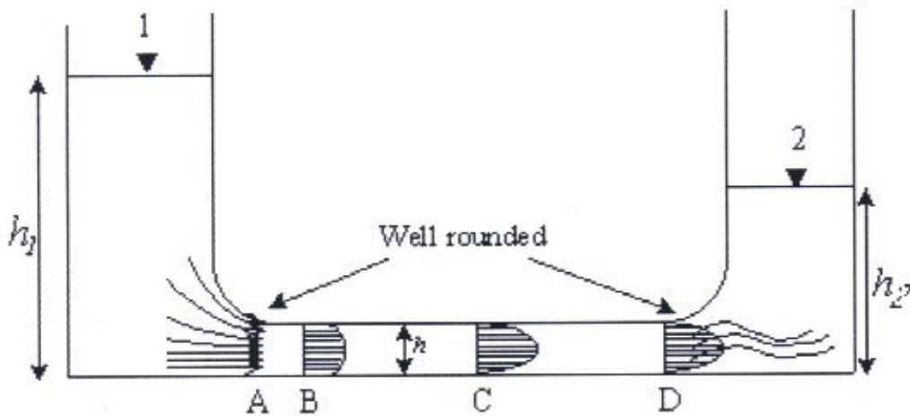
Assumptions:  $h_1 > h_2$ . The reservoirs are wide enough that the flow is quasi-steady. The two reservoirs have the same width, so that  $V_1 = V_2$ .
