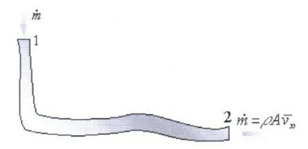
Note that according to continuity,  $\dot{m}$  is constant, so that the average velocity v increases when S becomes smaller.
