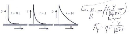
Supposed shape after scaling u with  $V_0$ , and y with a characteristic boundary layer thickness  $\delta$  that increases with time:
