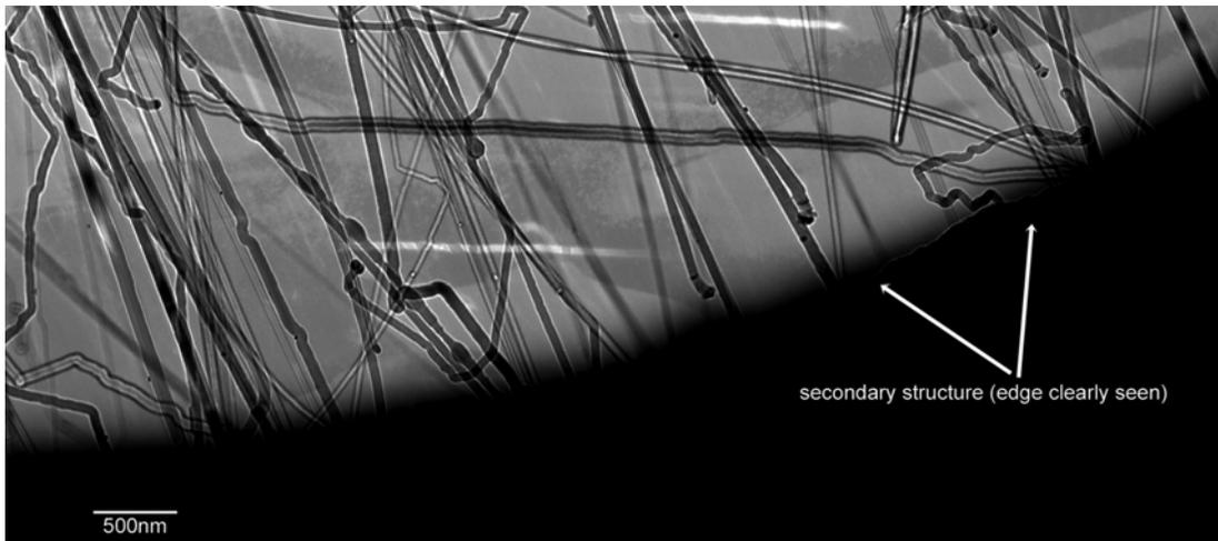
**Figure 5.5.** TEM imaging near edge of secondary structure. A micron long region clearly displays the edge with no shadowing. The level of kinking, bending and twisting near the tip appears to be reduced for nanowires contacting the secondary structure.
