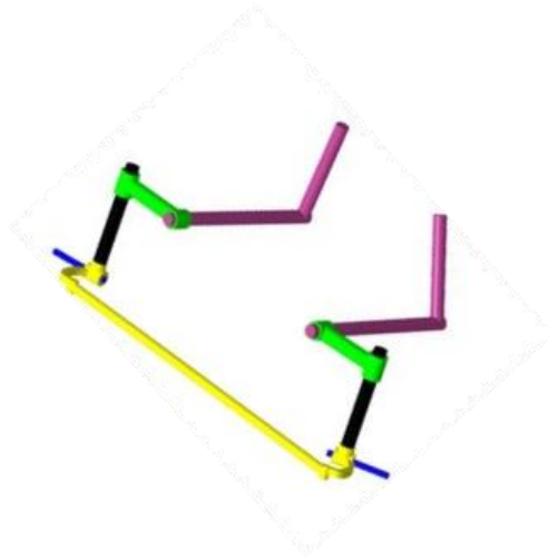
Figure 4: Steering mechanism assembly view.
