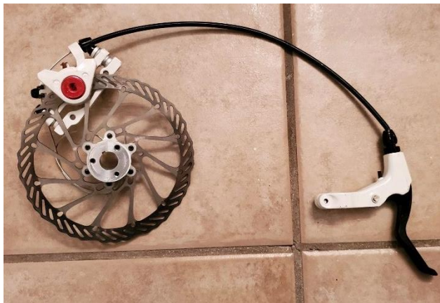
Figure 1.5.1 Disk brake and caliper trigger system.
