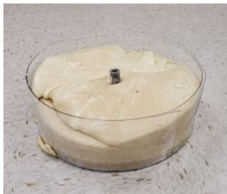
Figure 11: Wheel mold with expanding foam.
