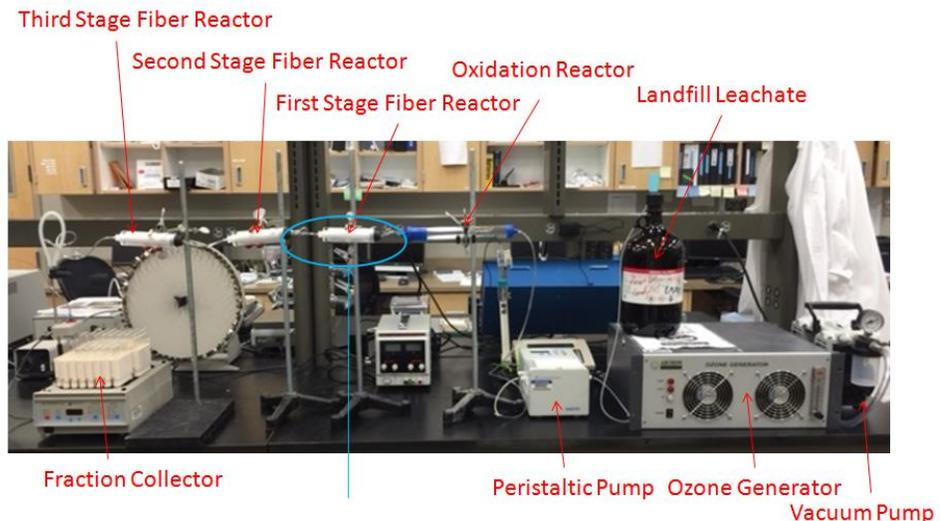
Figure 1. Experimental Setup
