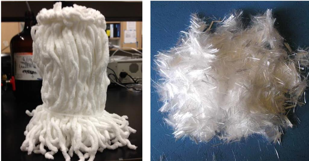
**Figure 13. Polypropylene Fibers used in Pressurized Biofilter**
