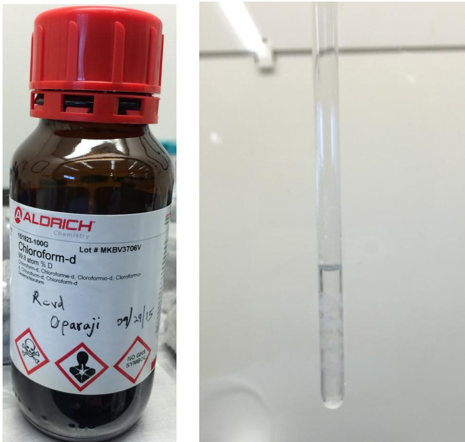
**Figure 34. Sample Preparation for NMR**
