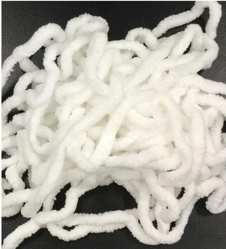
**Figure 2. Suspended Fiber Used for Biofiltration**
