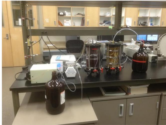
Figure 2. Recirculation Reactor and Fiber Reactor
