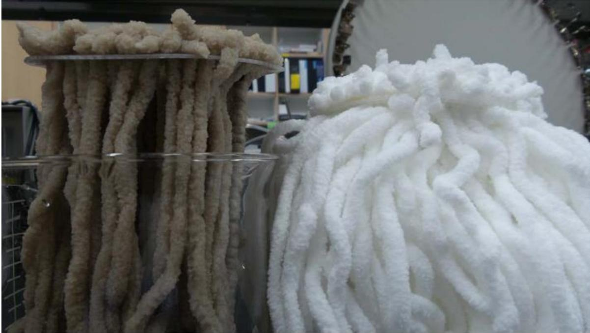
Figure 3. Polypropylene Fiber after (Left) and before (Right) Usage in the Pressurized Biofilter
