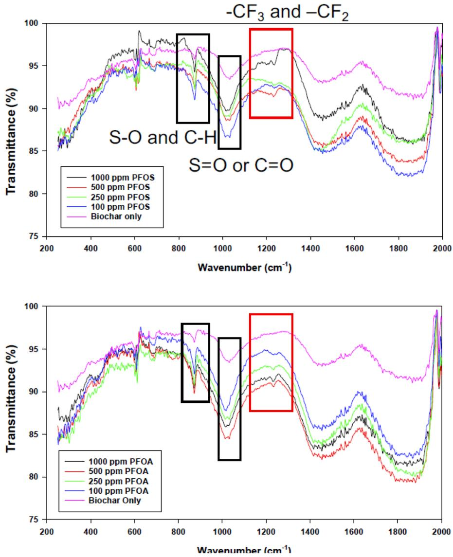
Figure 2. FTIR Analysis of PFOA and PFOS Adsorption on Engineered Biochar
