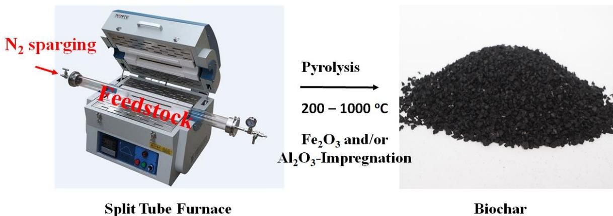
Figure 1. Biochar Synthesis Experimental Setup
