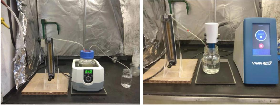
Figure 4. PFAS Sonochemical Degradation Experimental Setup
