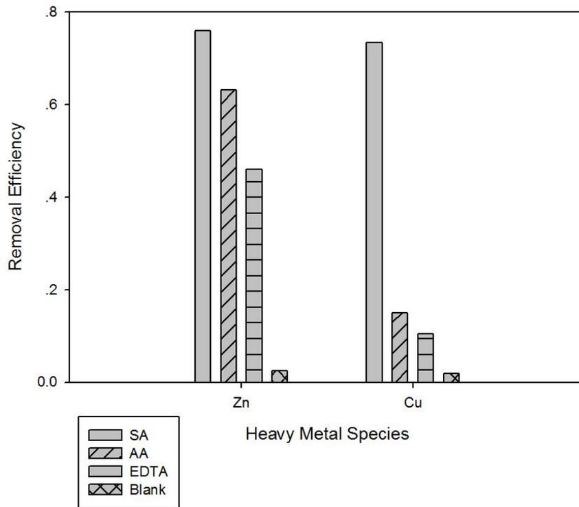
**Figure 1. Cu and Zn Extraction from Granular Sludge Pellet**
