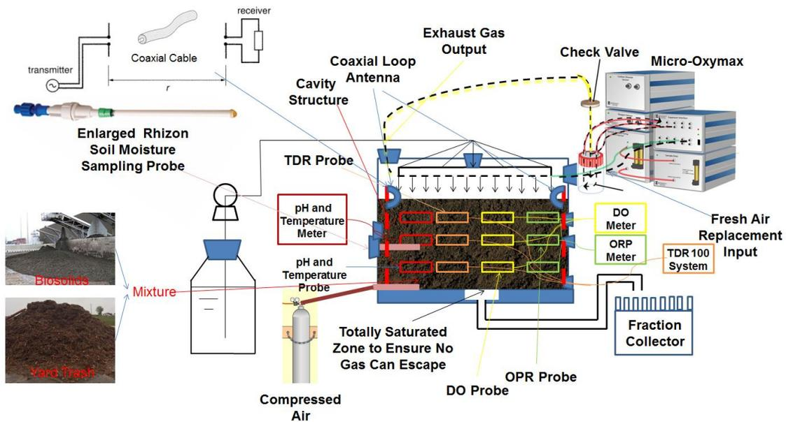
**Figure 2. Experimental Reactor Setup**
