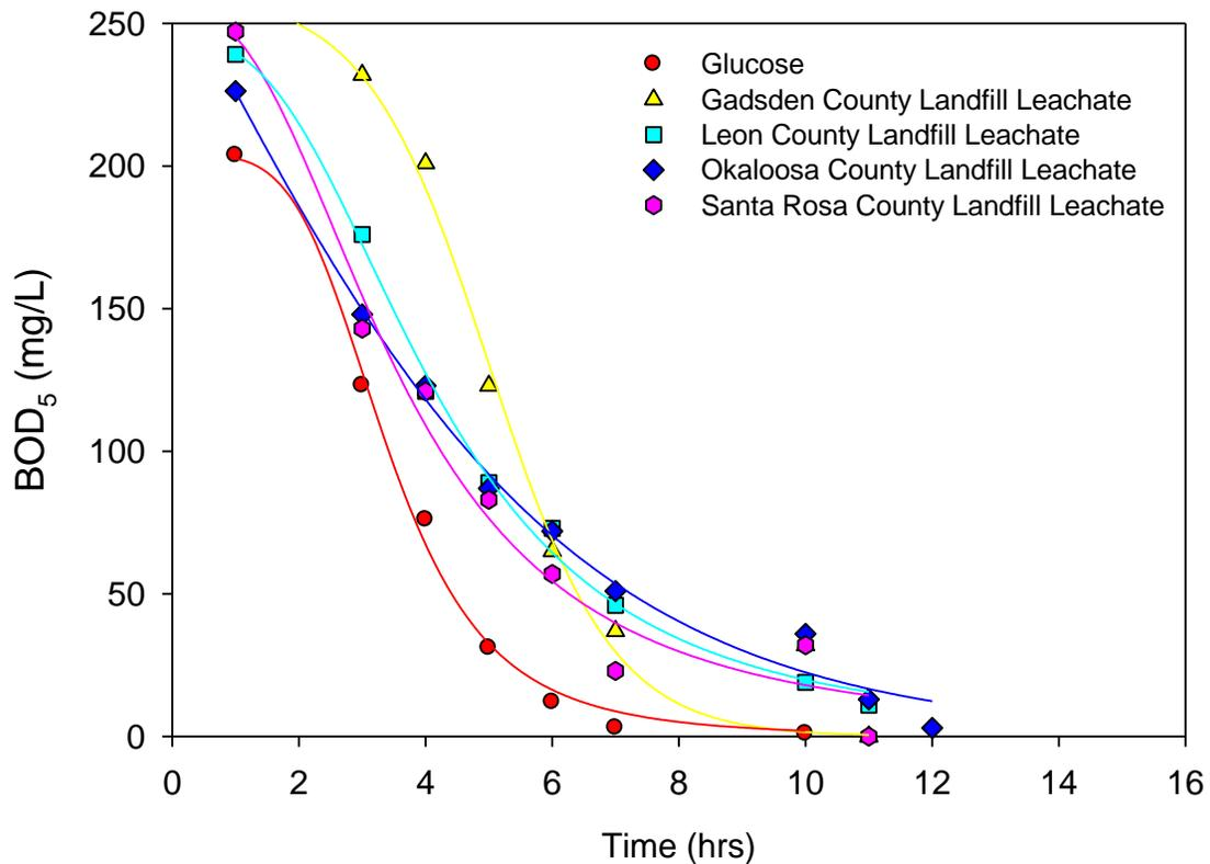
**Figure 24. Organic Decomposition in the Static MFC**
