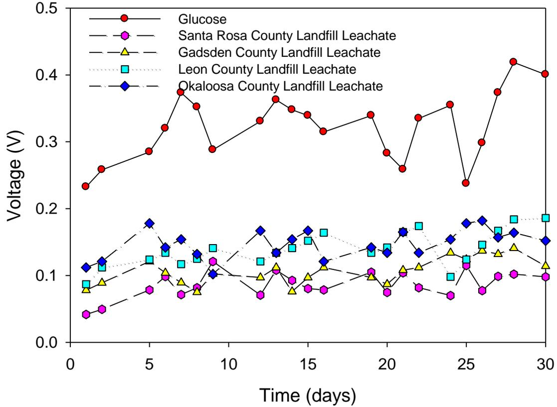
**Figure 15. Voltage Generation of the Continuous MFC**
