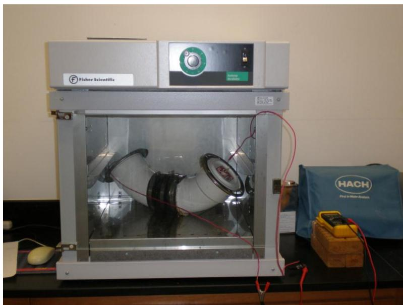
**Figure 13. Impact of Temperature on MFC Performance Setup**
