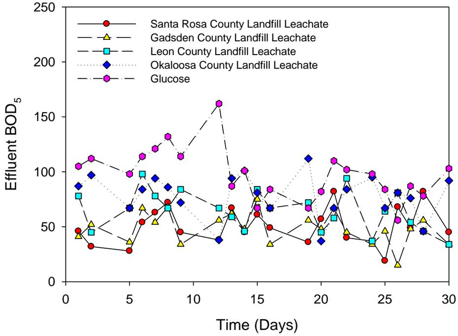
**Figure 16. Continuous MFC Effluent BOD<sub>5</sub> Values**
