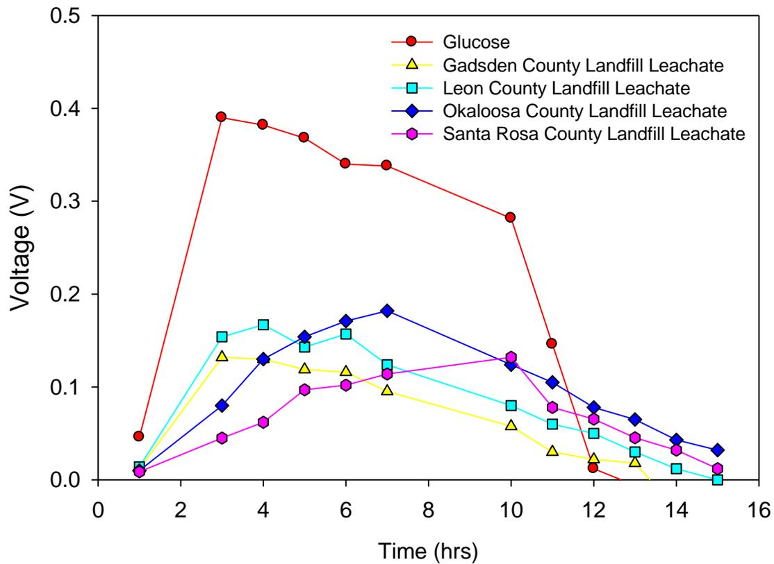
**Figure 14. Voltage Generation of the Static MFC**
