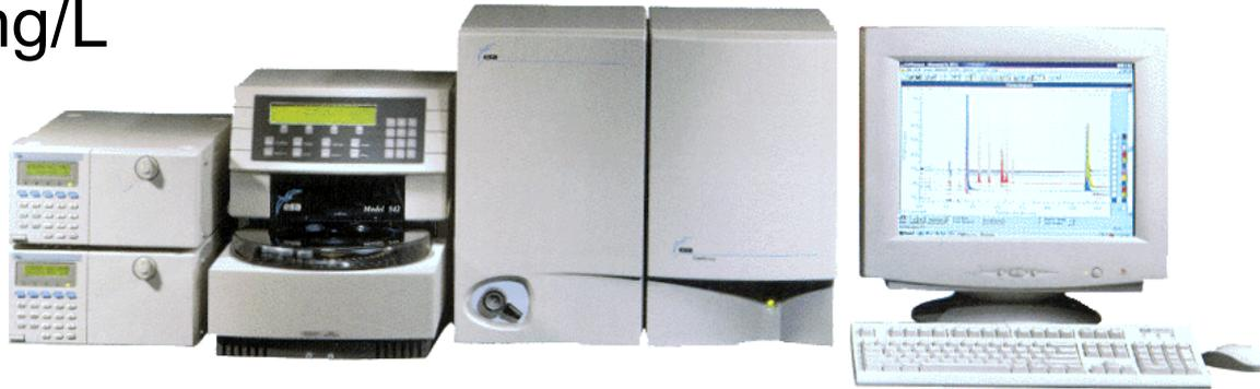
Benzene, toluene, *p*-xylene, PCE, and TCE to be monitored by a GC with a flame ionization detector and helium as the carrier gas
