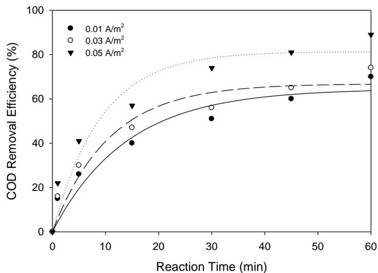
**Figure 2. Current Intensity and Time on COD Removal**
