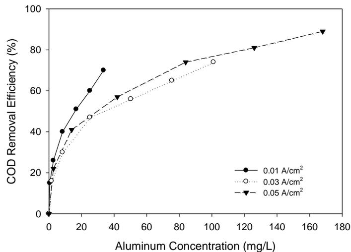
**Figure 4. COD Removal as a Function of Released Aluminum**
