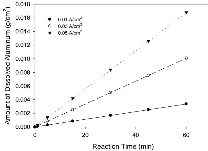
**Figure 3. Current Intensity and Time on Aluminum Dissolution**
