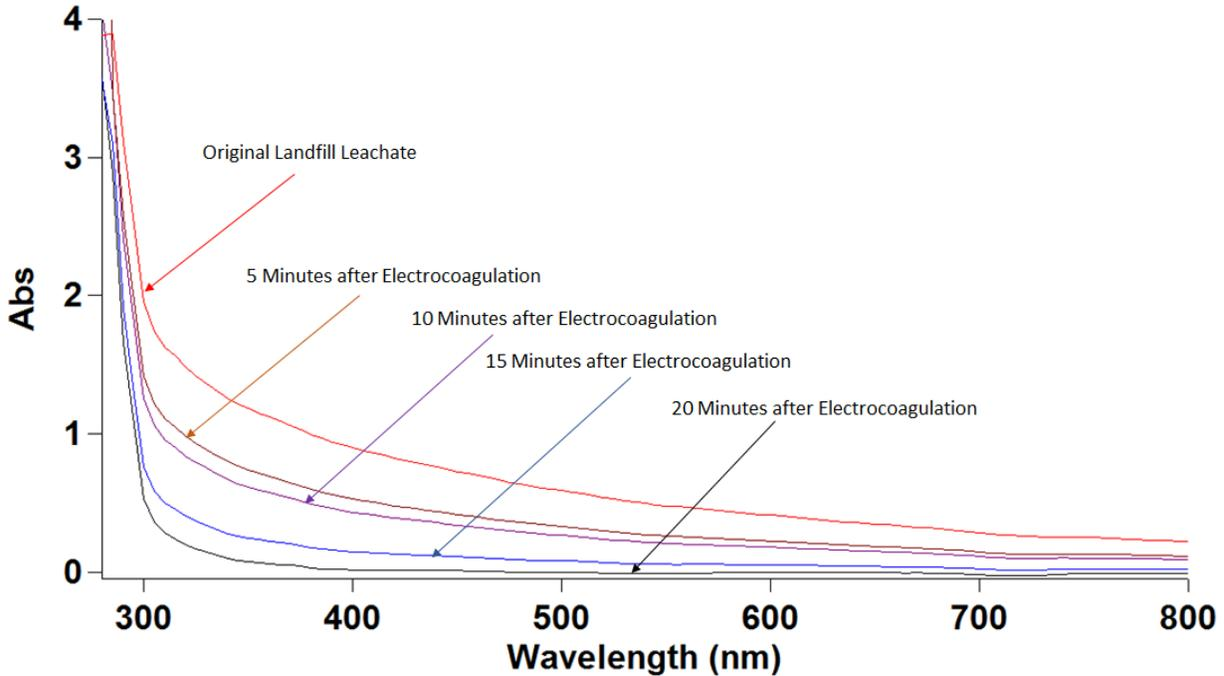
**Figure 2. Leachate UV-Vis Spectrum after Electrocoagulation**
