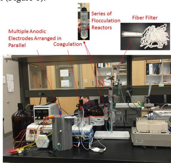
**Figure 1. Experimental Setup of This Research**
