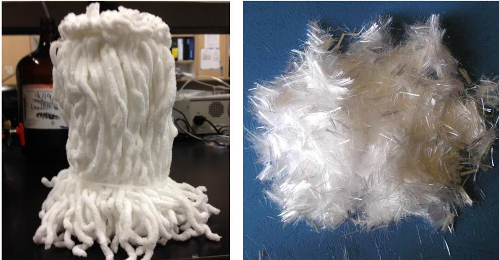
**Figure 2. Polypropylene Fibers Used in Biofilter**
