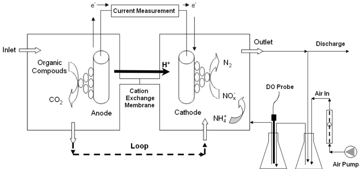
**Figure 1. MFC/Anammox Reactor Setup**
