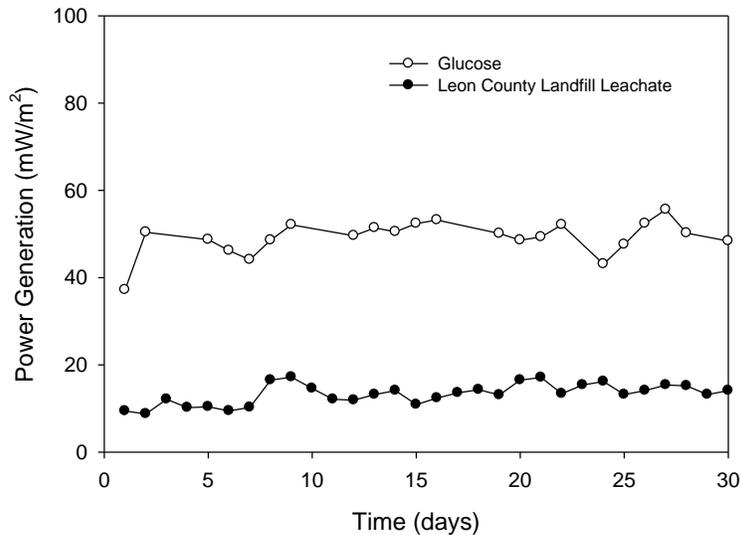
**Figure 2. Power Generation of the MFC/Anammox Reactor**
