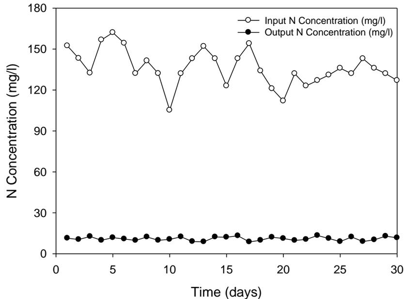
**Figure 3. Nitrogen Removal of the MFC/Anammox Reactor**
