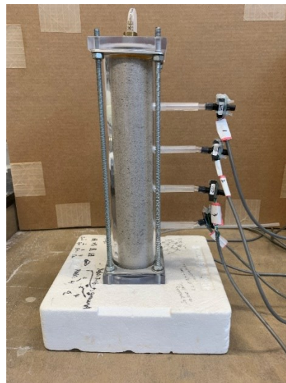
Figure 3. Unsaturated Column Experimental Setup
