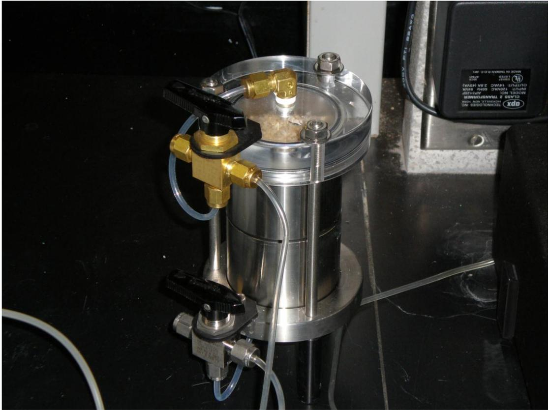
Figure 13. Filtration Column Assembly
