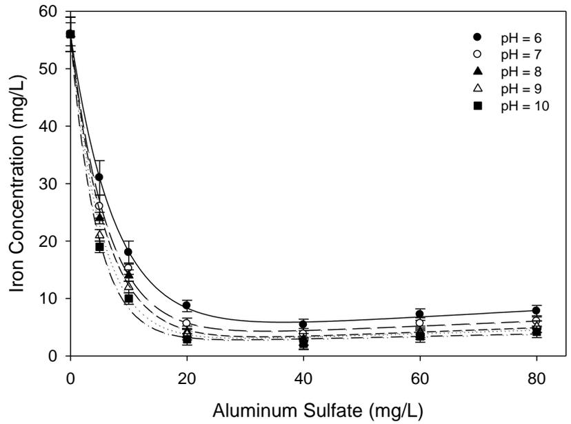
**Figure 4. Iron Removal as a Function of Alum Concentration**
