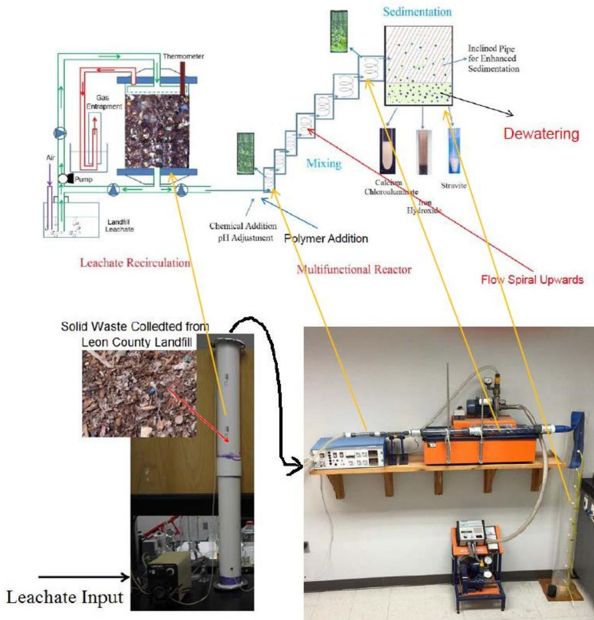
**Figure 1. Experimental Setup of This Research**
