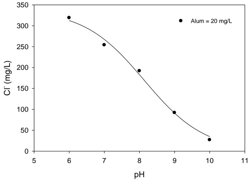
**Figure 3. Residual Chloride Concentration as a Function of pH**
