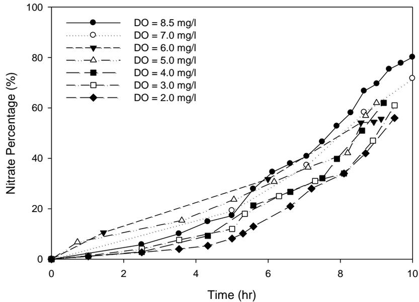
**Figure 4. Nitrate Production as a Function of Time**
