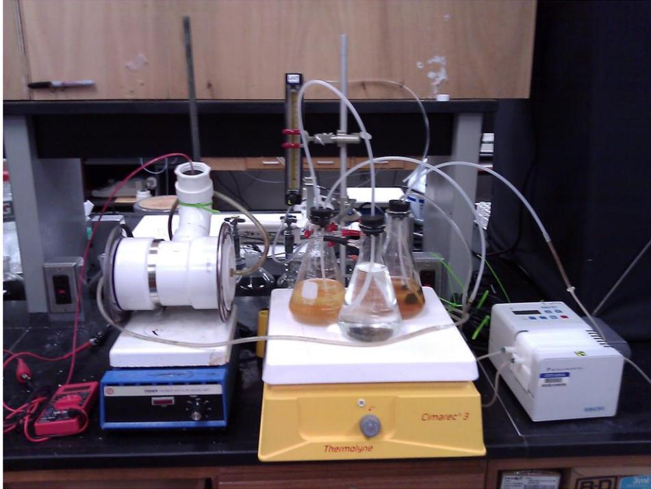
**Figure 2. Laboratory Setup for Ammonium Oxidation and MFC**
