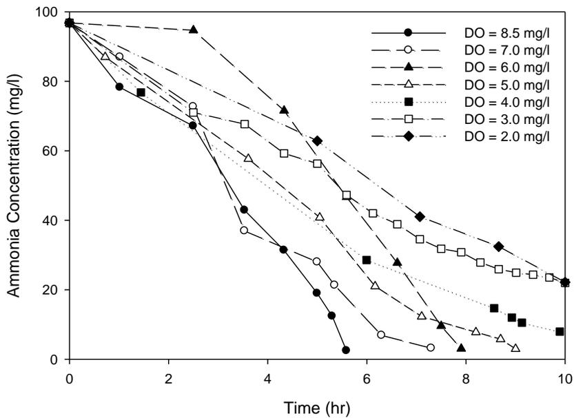
**Figure 3. Ammonia Depletion as a Function of Time**
