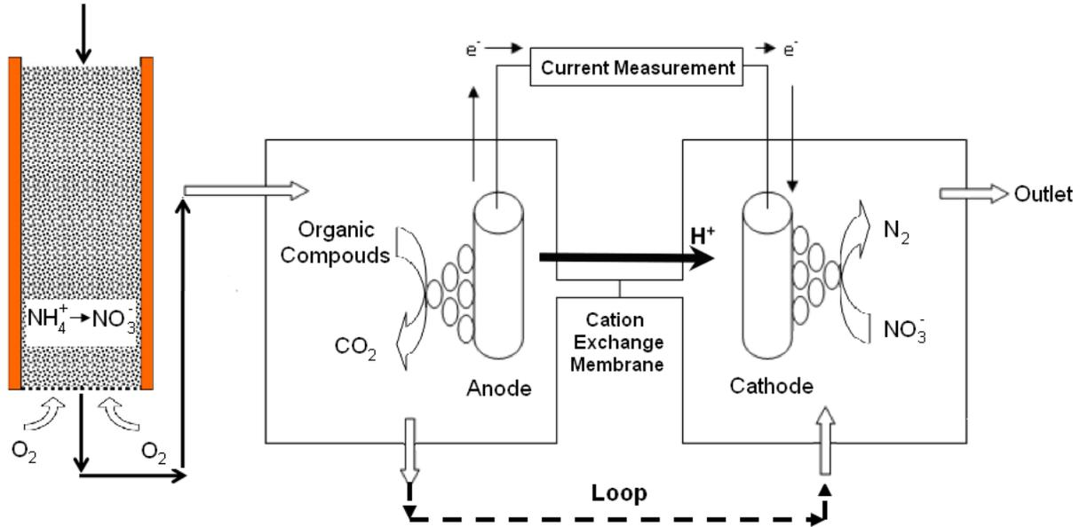
**Figure 1. Ammonium Oxidation/MFC Reactor Setup**
