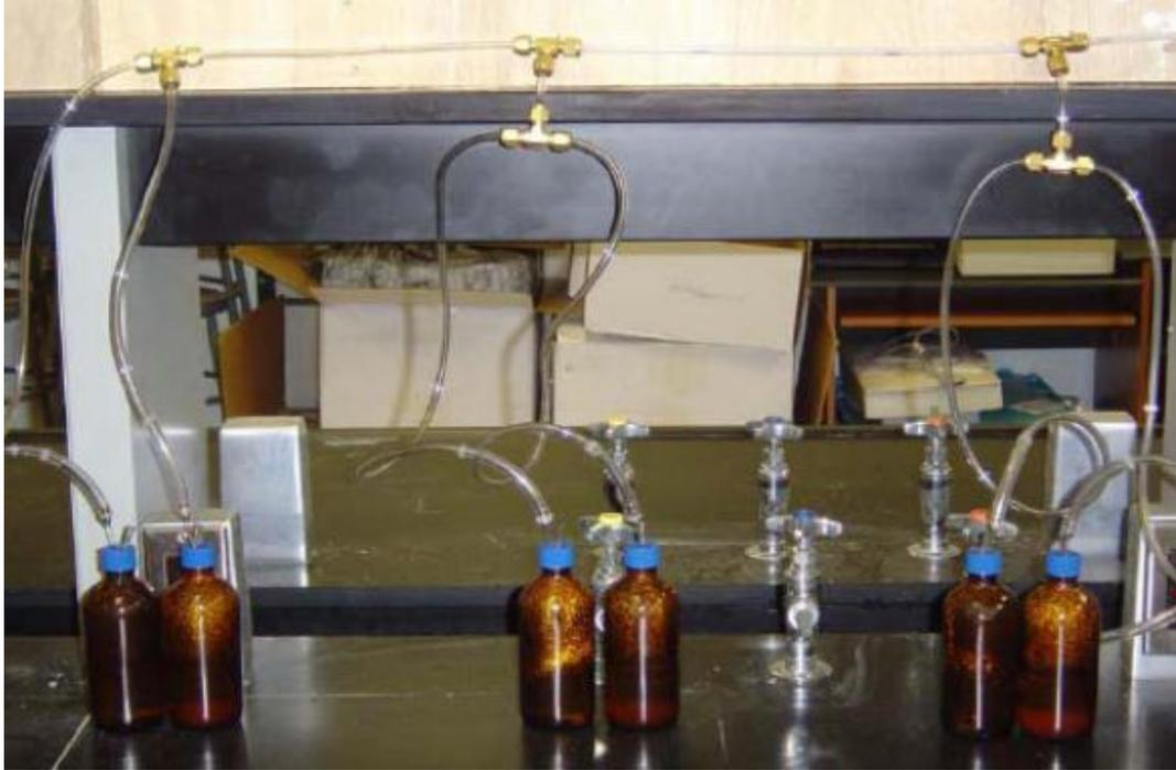
Figure 3. BTEX and TCE Biodegradation Experiment Setup
