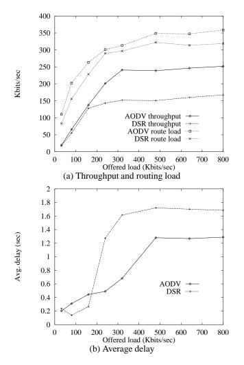
Fig. 8. Performance with increasing offered load with 100 nodes and 40 sources.
