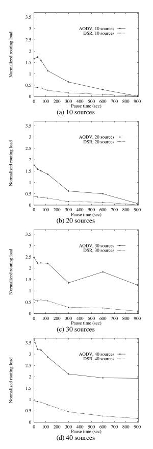
Fig. 3. Normalized routing loads for the 50 node model with various numbers of sources.
