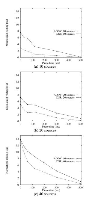
Fig. 6. Normalized routing loads for the 100 node model with various numbers of sources.
