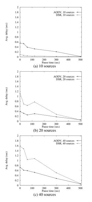
Fig. 5. Average data packet delays for the 100 node model with various numbers of sources.
