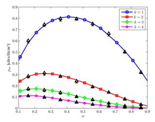
Fig. 3. Network secrecy rate density as a function of  $\alpha$  when the kth closest legitimate receivers are selected for b=2,  $\lambda_\ell=1$  [node/m²], and  $\lambda_e/\lambda_\ell=0.1$ . Lines represent analytical results. Black crosses and triangles represent the Monte Carlo simulations done for the case when interferer distances depend on the placement of the transmitters and for the case when interferer distances are generated independently, respectively.
