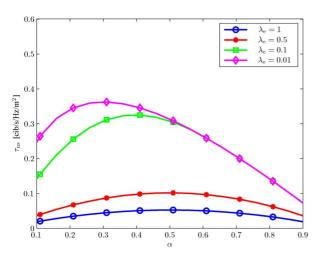
Fig. 7. Network secrecy throughput density as a function of  $\alpha$  when the closest legitimate receivers are selected for b=2,  $P_{\rm so}^*=0.1$ ,  $R_{\rm s}=4$  [cib/s/Hz],  $\lambda_\ell=1$  [node/m²], and different values of  $\lambda_{\rm e}$ .
