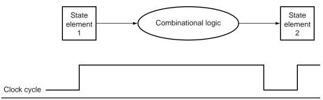
FIGURE B.7.2 The inputs to a combinational logic block come from a state element, and the outputs are written into a state element. The clock edge determines when the contents of the state elements are updated.
