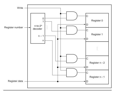
FIGURE B.8.9 The write port for a register file is implemented with a decoder that is used with the write signal to generate the *C* input to the registers. All three inputs (the register number, the data, and the write signal) will have set-up and hold-time constraints that ensure that the correct data is written into the register file.
