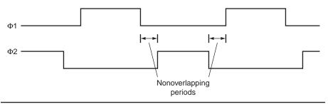
FIGURE B.11.3 A two-phase clocking scheme showing the cycle of each clock and the nonoverlapping periods.
