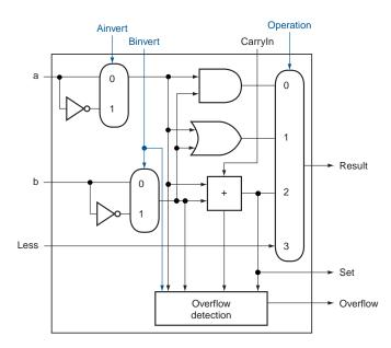
FIGURE B.5.10 (Top) A 1-bit ALU that performs AND, OR, and addition on a and b or  $\overline{b}$ , and (bottom) a 1-bit ALU for the most significant bit. The top drawing includes a direct input that is connected to perform the set on less than operation (see Figure B.5.11); the bottom has a direct output from the adder for the less than comparison called Set. (See Exercise 3.24 to see how to calculate overflow with fewer inputs.)
