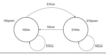
**FIGURE B.10.2** The graphical representation of the two-state traffic light controller. We simplified the logic functions on the state transitions. For example, the transition from NSgreen to EWgreen in the next-state table is  $(\overline{\text{NScar}} \cdot \text{EWcar}) + (\text{NScar} \cdot \text{EWcar})$ , which is equivalent to EWcar.
