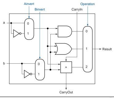
FIGURE B.5.9 A 1-bit ALU that performs AND, OR, and addition on a and b or  $\overline{a}$  and  $\overline{b}$ . By selecting  $\overline{a}$  (Ainvert = 1) and  $\overline{b}$  (Binvert = 1), we get a NOR b instead of a AND b.
