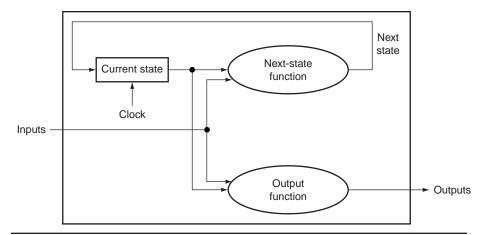
**FIGURE B.10.1** A state machine consists of internal storage that contains the state and two combinational functions: the next-state function and the output function. Often, the output function is restricted to take only the current state as its input; this does not change the capability of a sequential machine, but does affect its internals.
