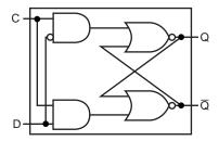
**FIGURE B.8.2** A D latch implemented with NOR gates. A NOR gate acts as an inverter if the other input is 0. Thus, the cross-coupled pair of NOR gates acts to store the state value unless the clock input, C, is asserted, in which case the value of input D replaces the value of Q and is stored. The value of input D must be stable when the clock signal C changes from asserted to deasserted.
