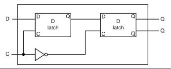
**FIGURE B.8.4** A **D flip-flop with a falling-edge trigger.** The first latch, called the master, is open and follows the input D when the clock input, C, is asserted. When the clock input, C, falls, the first latch is closed, but the second latch, called the slave, is open and gets its input from the output of the master latch.
