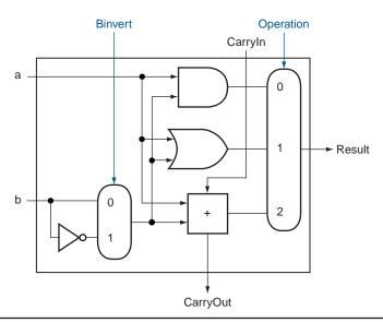
FIGURE B.5.8 A 1-bit ALU that performs AND, OR, and addition on a and b or a and  $\overline{b}$ . By selecting  $\overline{b}$  (Binvert = 1) and setting CarryIn to 1 in the least significant bit of the ALU, we get two's complement subtraction of b from a instead of addition of b to a.
