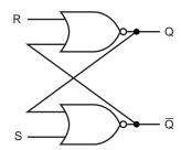
**FIGURE B.8.1** A pair of cross-coupled NOR gates can store an internal value. The value stored on the output Q is recycled by inverting it to obtain  $\overline{Q}$  and then inverting  $\overline{Q}$  to obtain Q. If either R or  $\overline{Q}$  are asserted, Q will be deasserted and vice versa.
