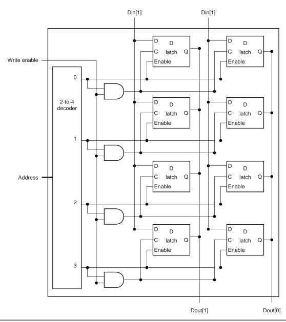
**FIGURE B.9.3** The basic structure of a 4 ¥ 2 SRAM consists of a decoder that selects which pair of cells to activate. The activated cells use a three-state output connected to the vertical bit lines that supply the requested data. The address that selects the cell is sent on one of a set of horizontal address lines, called the word lines. For simplicity, the Output enable and Chip select signals have been omitted, but they could easily be added with a few AND gates.
