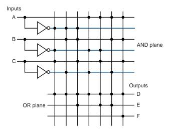
**FIGURE B.3.5** A PLA drawn using dots to indicate the components of the product terms and sum terms in the array. Rather than use inverters on the gates, usually all the inputs are run the width of the AND plane in both true and complement forms. A dot in the AND plane indicates that the input, or its inverse, occurs in the product term. A dot in the OR plane indicates that the corresponding product term appears in the corresponding output.
