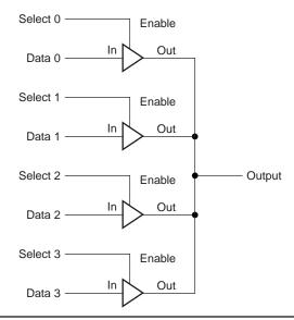
**FIGURE B.9.2 Four three-state buffers are used to form a multiplexor.** Only one of the four Select inputs can be asserted. A three-state buffer with a deasserted Output enable has a high-impedance output that allows a three-state buffer whose Output enable is asserted to drive the shared output line.
