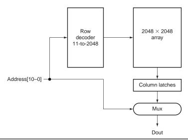
**FIGURE B.9.6** A 4M ¥ 1 DRAM is built with a 2048 ¥ 2048 array. The row access uses 11 bits to select a row, which is then latched in 2048 1-bit latches. A multiplexor chooses the output bit from these 2048 latches. The RAS and CAS signals control whether the address lines are sent to the row decoder or column multiplexor.
