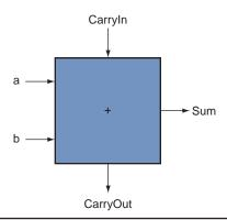
**FIGURE B.5.2 A 1-bit adder.** This adder is called a full adder; it is also called a (3,2) adder because it has 3 inputs and 2 outputs. An adder with only the a and b inputs is called a (2,2) adder or half adder.
