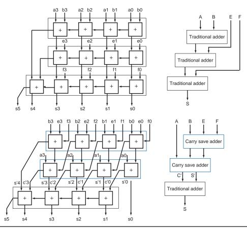
**FIGURE B.14.1 Traditional ripple carry and carry save addition of four 4-bit numbers.** The details are shown on the left, with the individual signals in lowercase, and the corresponding higher-level blocks are on the right, with collective signals in uppercase. Note that the sum of four n-bit numbers can take n + 2 bits.
