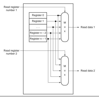
**FIGURE B.8.8** The implementation of two read ports for a register file with *n* registers can be done with a pair of *n*-to-1 multiplexors each 32 bits wide. The register read number signal is used as the multiplexor selector signal. Figure B.8.9 shows how the write port is implemented.
