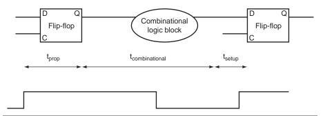
FIGURE B.11.1 In an edge-triggered design, the clock must be long enough to allow signals to be valid for the required set-up time before the next clock edge. The time for a flip-flop input to propagate to the flip-flip outputs is  $t_{\rm prop}$ ; the signal then takes  $t_{\rm combinational}$  to travel through the combinational logic and must be valid  $t_{\rm setup}$  before the next clock edge.
