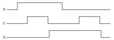
**FIGURE B.8.5** Operation of a D flip-flop with a falling-edge trigger, assuming the output is initially deasserted. When the clock input (C) changes from asserted to deasserted, the Q output stores the value of the D input. Compare this behavior to that of the clocked D latch shown in Figure B.8.3. In a clocked latch, the stored value and the output, Q, both change whenever C is high, as opposed to only when C transitions.
