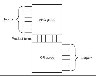
**FIGURE B.3.3** The basic form of a PLA consists of an array of AND gates followed by an array of OR gates. Each entry in the AND gate array is a product term consisting of any number of inputs or inverted inputs. Each entry in the OR gate array is a sum term consisting of any number of these product terms.
