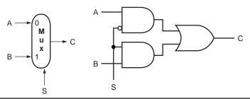
**FIGURE B.3.2** A two-input multiplexor, on the left, and its implementation with gates, on the right. The multiplexor has two data inputs (A and B), which are labeled 0 and 1, and one selector input (S), as well as an output C. Implementing multiplexors in Verilog requires a little more work, especially when they are wider than two inputs. We show how to do this beginning on page B-23.
