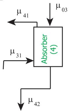
There are 4 degrees of freedom: P, T, key component recovery and liquid feed rate.
