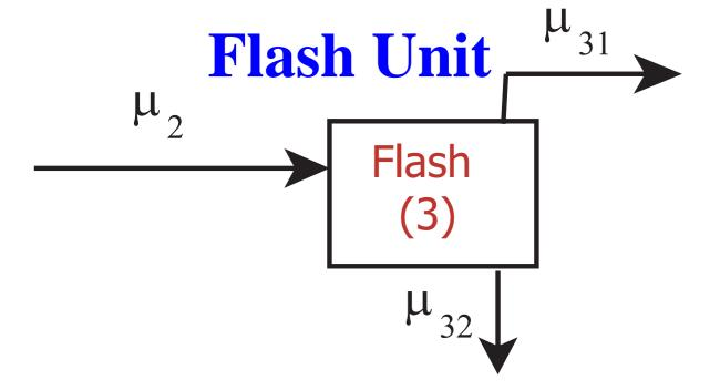
Assume a pressure drop of  $0.5\ bar$  from the reactor and operate the flash at  $68.5\ bar$ .
