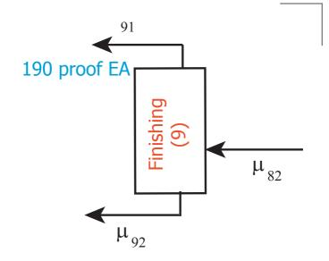
This last column is used to obtain the ethanol product at the azeotropic composition
