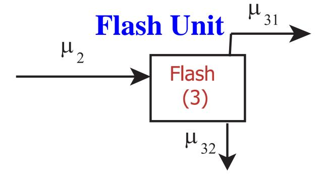
We want to take the reactor effluent to cooling water temperature and separate the liquid product from reactants.
