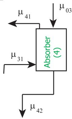
There are 4 degrees of freedom: P, T, key component recovery and liquid feed rate.
