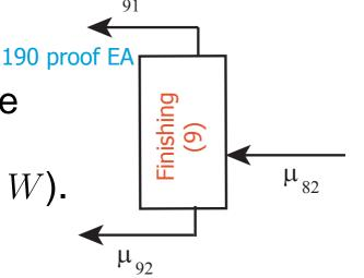
This last column is used to obtain the ethanol product at the azeotropic composition (85.5% EA and 14.5% W).
