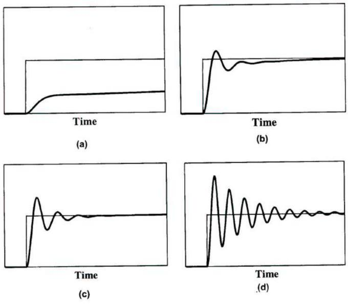
Figure 7.1 Control response for a setpoint change. (a) Controller tuned for sluggish response. (b) Controller tuned for 1/10 decay ratio. (c) Controller tuned for QAD. (d) Controller tuned for ringing response.
