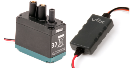
FIGURE 10: Motor (Left) & Controller (Right)
