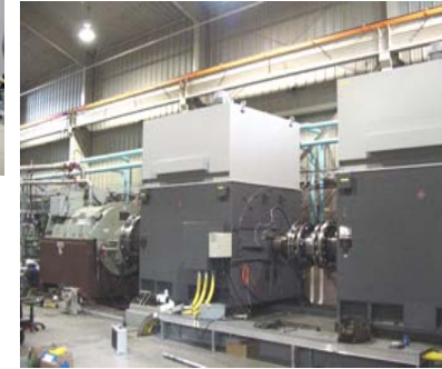
5 MW advanced prototype test facility for motors, converters, transformers.
