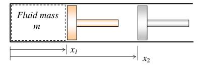
Consider a fluid mass m going through an expansion process from  $x_1$  to  $x_2$ . The system is identified as the fluid mass m enclosed by the dashed region inside the cylinder.
