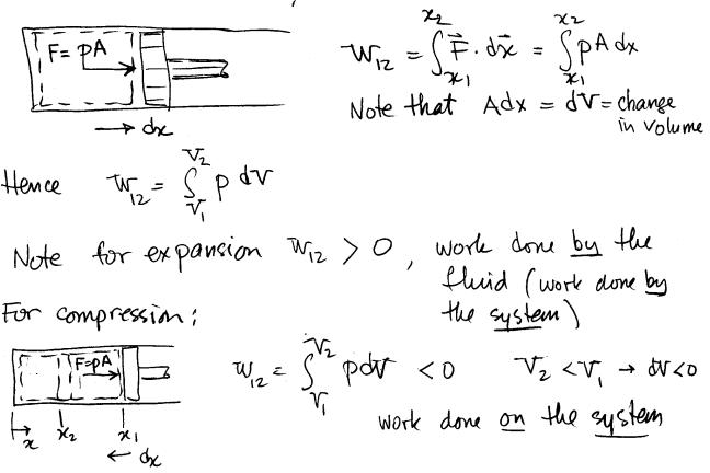
Note that in this example, the mass of the system remained unchanged, throughout the process. Such a system is called a
