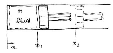
Consister a fluid of mass m going through an expansion process from x, to Xz. The system is identified as the fluid mass m enclosed by the deshed line inside the cylinder. The fluid exerts a force on the piston, and maves the piston in the positive x direction. The force exerted is F=pA
