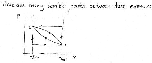
The objective is to connect processes to create a CYCLE. There are many ways to create a cycle between Vmin and Vmax
