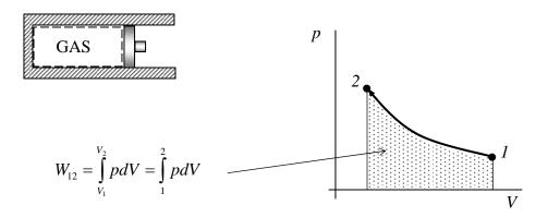
To evaluate this integral, we must have an expression for p as a function of V. A relationship among the p, V, and T variables is called an **equation of state**. We shall now obtain the expressions for work for each of the four processes of the Stirling engine.
