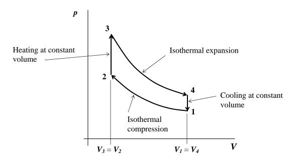
We shall now compute the work for each of the processes and for the cycle as a whole.
