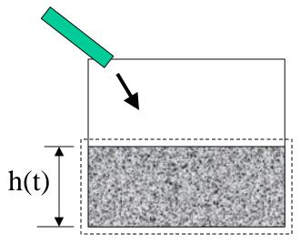
Water is fed into an empty tank using a hose of cross-sectional area of 0.0005 m<sup>2</sup>. The flow speed out of the hose is measured to be 10 m/s. Determine the rate of increase for the water height inside the tank dh/dt. The cross-sectional area of the tank is 1 m<sup>2</sup>.
