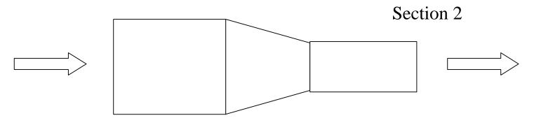
Air flows through a converging duct as shown. The areas at sections 1 & 2 are 5  $\text{m}^3$  and 1  $\text{m}^3$ , respectively. The inlet flow speed is 20 m/s and we know the outlet speed at section 2 is 100 m/s by mass conservation. If the pressure at section 2 is the atmospheric pressure at  $1.01 \times 10^5 \, \text{N/m}^2$ , what is the pressure at section 1. Neglect all viscous effects and given the density of the air
