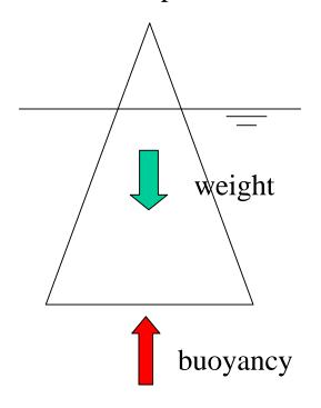
When the iceberg floats, its weight balances the buoyancy force exerted on the iceberg by the displaced water.
