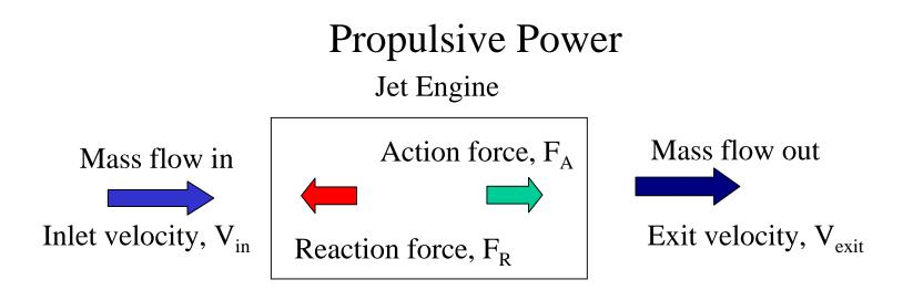
Due to the action force  $F_A$ , the momentum of the air flowing through the engine increases:
