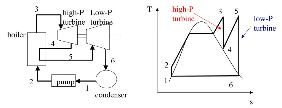
We are going to add a low pressure turbine (5-6) to the system we just analyzed. Before going into the L-P turbine, the exit steam from the first turbine (3-4) is reheated in the boiler at a constant pressure. Assume both 4 & 6 are at 100% saturated vapor state and the vapor exiting from the H-P turbine (state 4) expands to a lower pressure of 2 MPa (P<sub>4</sub>=2 MPa) before it is being reheated at a constant pressure to the state 5. Recalculate (a) the thermal efficiency of the system.
