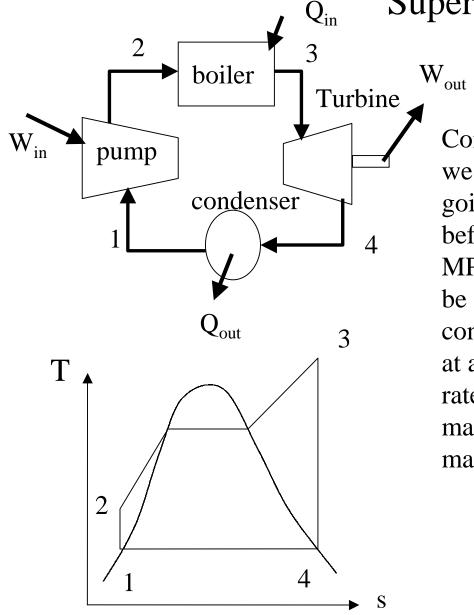
Consider the same Rankine power cycle as we analyzed before. But this time we are going to superheat the steam in the boiler before allowing it to enter the turbine at 6 MPa. The steam exits from the turbine will be 100% saturated vapor as shown. After condensing, saturated liquid enters the pump at a pressure of 0.1 MPa. Determine (a) the rate of heat transfer into the boiler per unit mass, (b) the net power generation per unit mass. (c) the thermal efficiency,
