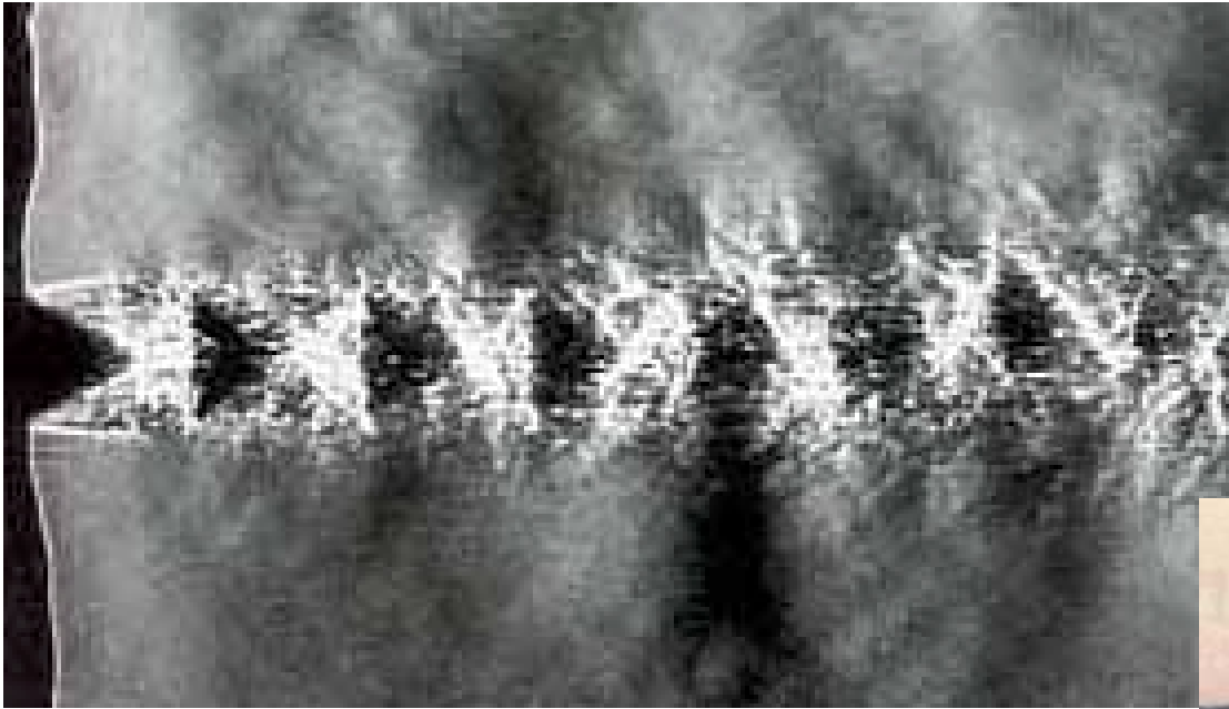
An under-expanding jet visualized by shadowgraph
