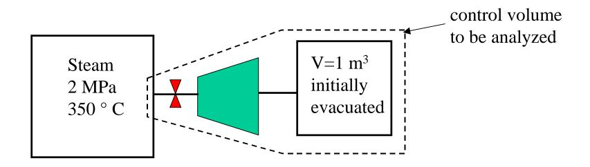
Assumptions: dQ/dt=0 adiabatic process, KE and PE are negligible Steam properties at the first tank remains constant The second tank reaches final equilibrium after the filling process ends Mass conservation
