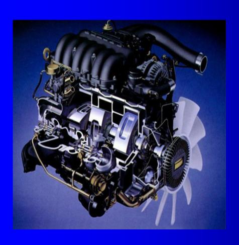
New triple rotor engine in development by Mazda Corp.
